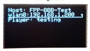
Pressing the button on the right, labeled Enter, while the OLED display is on the Standby screen will open the Status Screen.
