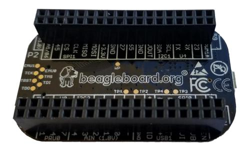
The pins are very close so take extreme caution that you don't have any solder bridges. It is recommended to test each pin to make sure.
