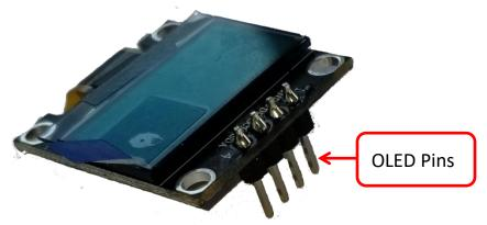
Press the OLED Display onto the F8-PB insuring that all four pins are fully inserted into the header and oriented like the picture below:
