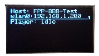
If you press the button on the left, labeled Test/Down, while the OLED display is on the Standby screen then the F8-PB will go into test mode and output a test pattern to the **configured** output ports. It will display alternating test patterns. It will cycle through a Red-Green-Blue cycle then go to a Red-Green-Blue-White-Off cycle and then turn off and then cycle again. The OLED will show the FPP in testing mode.
